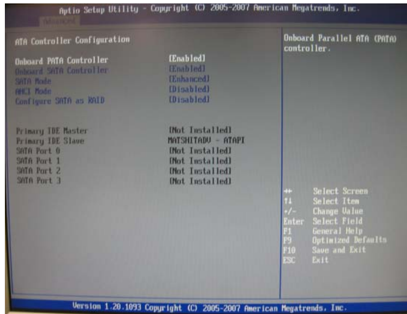
Figure 5-41 ATA Controller Configuration
